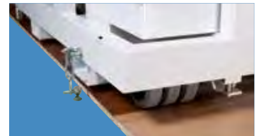
Alternative tie-down system (optional): 1 anchor on each side of base frame.
