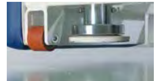
Pedestal feet retract automatically as unit is lowered to storage position.
